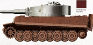
2. Hull with application of anti-rust red primer "red primer" based on lead, the turret has not been painted due to a lack of anti-rust product.
