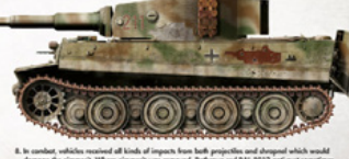
8. In combat vehicles received all kinds of impacts from both projectiles and shrapnel which would damage the armor. When armor was removed, RAL 8017 anti-rust sometimes appeared. In other instances, this is not the case, as the absence of red anti-rust on the turret means the light grey of the paragonizing treatment appears.
