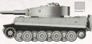
1. Hull and turret of a Tiger I after the anti-rust treatment called paragonizing using zinc phosphorus.
