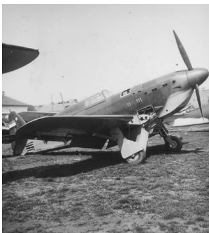
Damaged Rogožarski IK-3 Br.13/No13-2162 captured at Zemun airfield, april 1941. Nice view on enlarged flaps detail. Short UC leg cover. Photo - Jan Vd Heuvel collection via Nenad Miklušev
